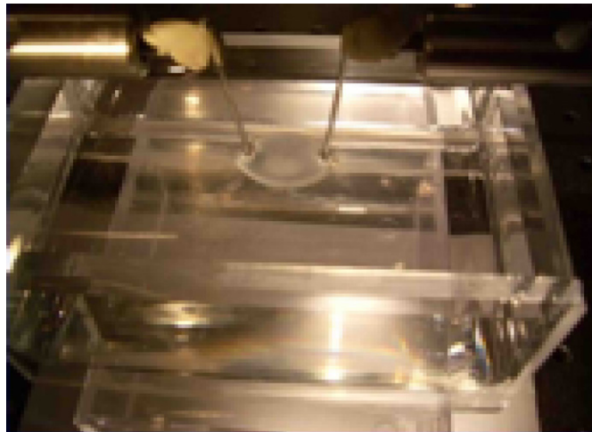
Figure 6. Experimental set up. A circular film of mineral oil was floated on water. Metal pins extended only into the oil film and not into the water below. The pins were connected to electronic micrometers to apply traction in the 180^\circ meridian.
